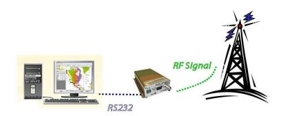
RS-232 serial cables are very limited on how long they may be run, so the RV-M7 transceiver must be physically close to the PC running the AVL software.
