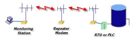
Incorporated in the radio is a built in store-and-forward repeater function. The repeater function works only in the Packet Mode, and will not repeat streaming messages. A repeater can extend the range of a system by 2-20X, depending upon how high-up above the average terrain the repeater is mounted.
