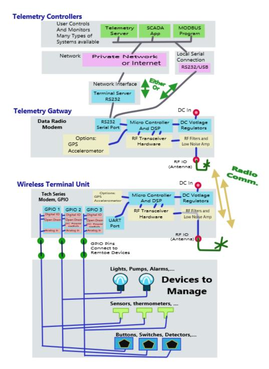
The **IOPIN** command is used to configure the functions of the GPIO pins. **IOPIN XX M** command set the GPIO IO pins on the Tech Series GPIO front panel to inputs or outputs.
