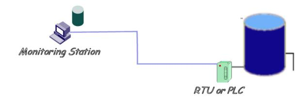
When the distance between the monitoring station and the device being monitored (the water tank above) is not trivial, than a wireless link between the two sites becomes a logical means of connecting them.
