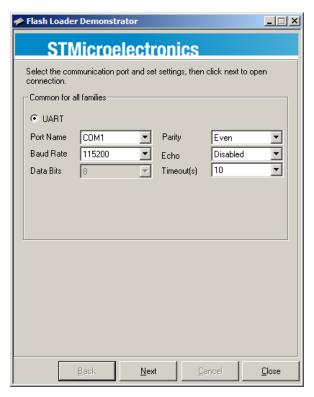
Select the serial port connected to the M8 and leave the other options at their default value. Click Next. The screen below should appear. If instead an error is shown, check wiring and ensure no lights are flashing on the M8. If lights are flashing, it is an indication that the boot loader was not correctly entered.
