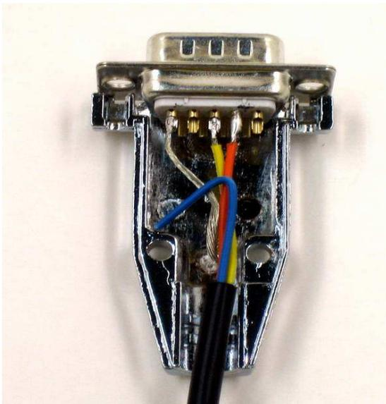
The **orange wire** goes to pin two of the DB9, the **yellow wire** to pin 3, and the shield braid of the cable connects to pin 5 of the DB9. The blue wire is trimmed off.
