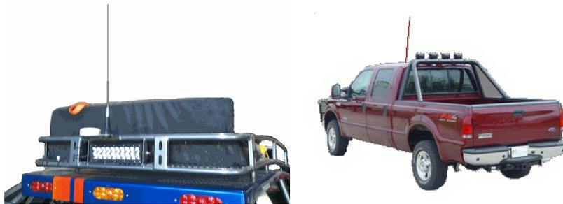
Avoid using magnet-mount antennas for race vehicles. They may be OK for a chase vehicle if the driving and terrain is not too rough.
