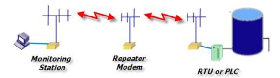
Incorporated in all Raveon Data Radio Modems is a *store-and-forward repeater* function.
