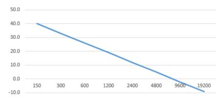
As you can see, 9.6GHz is 40dB lower than 150MHz. 40/6 = 6.6 so 150Mhz signals are 6.6 times longer range than 9.6GHz.
