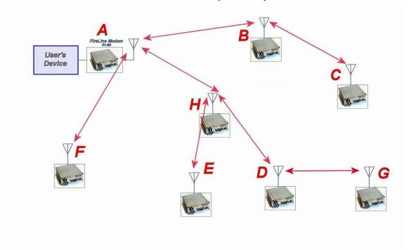
In the example shown in Figure 3 above, *RADIO* A is will communicate with all other modems in the system. It can directly communicate with B, H, and F. Because of propagation limits, it cannot communicate reliable to E, D, C, and G.
