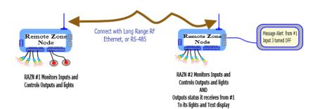
servers, or simple to a graphical display. Many different versions of the RAZN have analog inputs, and the RV-N55-7 version has the ultra-high resolution ADC in it that is the ideal device to monitor a Thermocouple Sensor.
