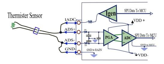
Resistor temperature sensors definitely need current put into them, and some Thermocouple sensors have used current powering them.
