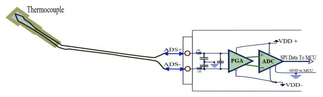
Raveon's Remote Autonomous Zone Node (RAZN) has delta-sigma analog-to-digital converters (ADCs) are ideal data converters for measuring, monitoring, and reporting thermocouples.
