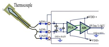
may not be the same as the RAZN ground. This can cause a variety of problems so don't ground if this won't work for your system, and when not grounded ensure that lighting or large voltage spikes won't hit the thermocouple. When using an exposed or grounded thermocouple, ensure that the thermocouple contact does not disrupt signals.
