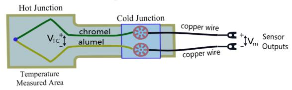
The two Cold Junction connections should be made at the same temperature. The Cold Junctions are mounted on an isothermal block of high thermally conductive material. If the Cold Junction was at 0°C then Sensor Output would be zero volts and we would be able to measure the hot junction voltage directly.
