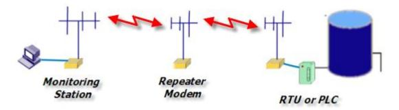
Incorporated in the radio is a built in store-and-forward repeater function. The repeater function works only in the Packet Mode, and will not repeat streaming messages. A repeater can extend the range of a system by 2-20X, depending upon how high-up above the average terrain the repeater is mounted.
