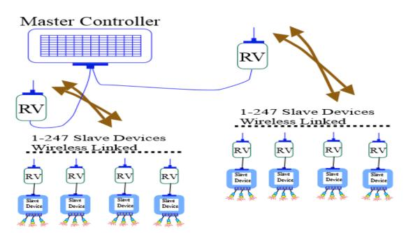
If millions of Slaves need to be accessed with Modbus, Modbus can access millions of devices over radio waves, and Raveon's Cigorn Gateway can route the Modbus messages to the correct base station for millions of devices.
