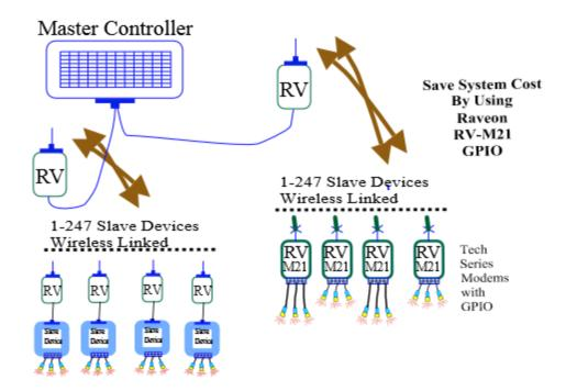
Most MODBUS slave devices can only report when queried. All Raveon SCADA slaves can respond to MODBUS inquiries and can have their registers and IOs managed by the Master Controller. The RV-M21 and RV-M22 radio modems have General Purpose IO (GPIO) SCADA IO pins built into the modems and the Flexible Digital IO (FIO) option has 8 TTL IO pins with SCADA features for digital inputs or outputs.
