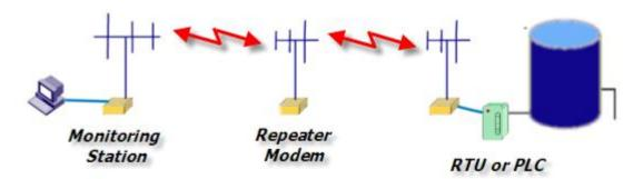
Incorporated in all Raveon Data Radio Modems, where allowed by regulation, is a **store-and-forward repeater** function. The repeater function works in the Packet Mode. A repeater can extend the range of a system by 2-20X, depending upon how high-up above the average terrain the repeater is mounted. Repeater systems are often 100 to 500 square miles per repeater.
