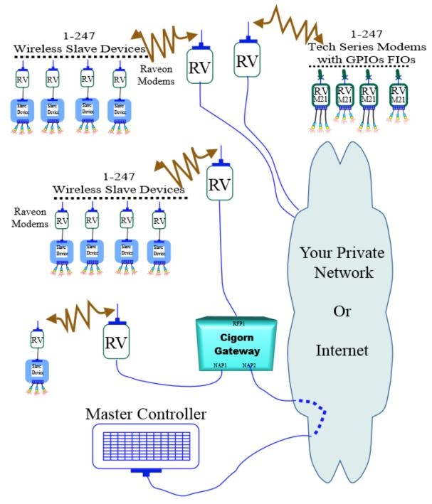
The Raveon data radio modems shown above (RV) can be used as the base stations and as the modems for the SCADA devices. The Cigorn can be configured to route as you want, so dozens of base stations can be used, talking to even millions of radio modems or slave devices.
