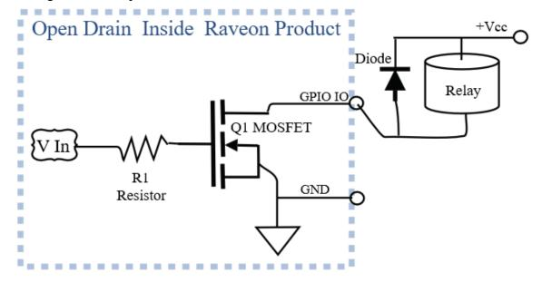
Use Open Drain for enabling: Lights, Relays, LEDs, Valves, AC power switches ...
