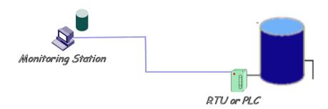
When the distance between the monitoring station and the device being monitored (the water tank above) is not trivial, than a wireless link between the two sites becomes a logical means of connecting them. The RTU monitors the digital and analog parameters in the field, and transmits data to the central Monitoring Station using a SCADA protocol.
