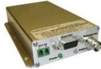
Although it features plug-and-play operation, working straight out of the box as a point-to-point or point-to-multipoint radio modem, the user may configure it for more advanced network topologies, repeating, and diagnostic abilities.
